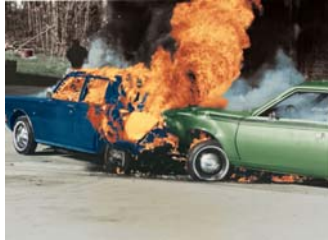
Fuel tank integrity
